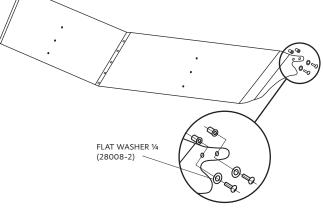
$^{\ast}$  Depending on the year of the truck, holes may need to be drilled on the front of the cab for proper installation
