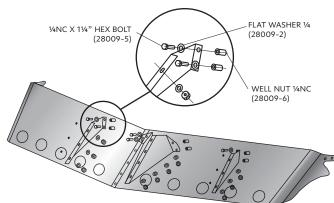
6. Fasten the sides of the sun visor to the cab with original screws. Feed the original screws and ¼ flat washer through each of the 4 holes. Tighten with the original well nuts.
