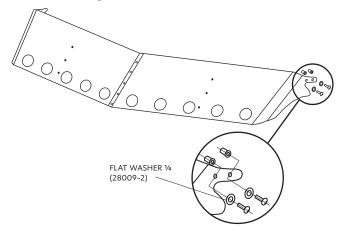
\* Depending on the year of the truck, holes may need to be drilled on the front of the cab for proper installation
