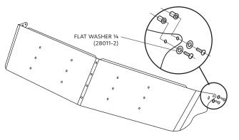
\* Depending on the year of the truck, holes may need to be drilled on the front of the cab for proper installation
