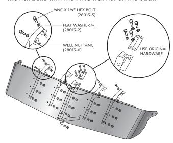
6. Fasten the sides of the sun visor to the cab with the original sunvistor hardware. Feed the screw and flat washer through each of the 4 holes. Tighten with the original well nuts.
