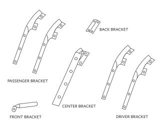
4. Fasten each screw to all brackets with a ¼ lock washer and ¼ hex nut on the back side of the bracket.
