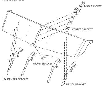
5. Attach the brackets to the cab with the ¼NC x 1¼" hex bolt. Feed the ¼NC x 1¼" hex bolt and a ¼ flat washer through each hole of the bracket. Fasten the hex bolts with the ¼NC well nut on the back.
