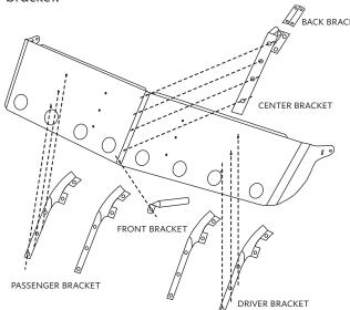
5. Attach the brackets to the cab with the ¼NC x 1¼" hex bolt. Feed the ¼NC x 1¼" hex bolt and a ¼ flat washer through each hole of the bracket. Fasten the hex bolts with the ¼NC well nut on the back.
