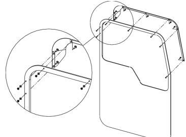
Driver side shown, use reverse orientation for passenger side
