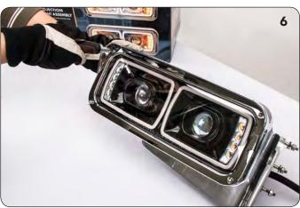
Special Installation Note: If fuse blows on high beam, please flip the high beam plug over 180 degrees.
