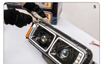
**6.** Install the outer bezel with the visor at top using the 4 screws removed in step 1.
