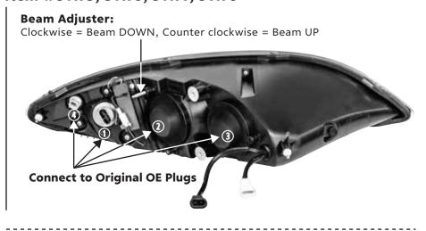
The **Brown** Positive Wire for the LED position light must NOT be hooked into any of the OE harnesses. It is recommended this Brown Positive Wire be hooked to a 12v + source independent of the OE light harnesses. Locate a power wire which activates an accessory (e.g. dash auxiliary) when the ignition is in the "ON" position, so that the LED position light only comes on when the truck ignition is "ON" and running.
