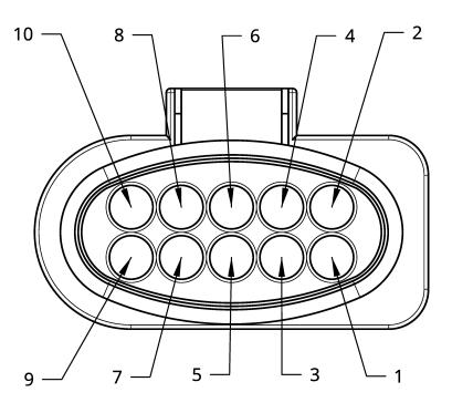
NOTE: VIEW FROM BACK OF VEHICLE'S EXISTING HEADLIGHT WIRING HARNESS MALE CONNECTOR
