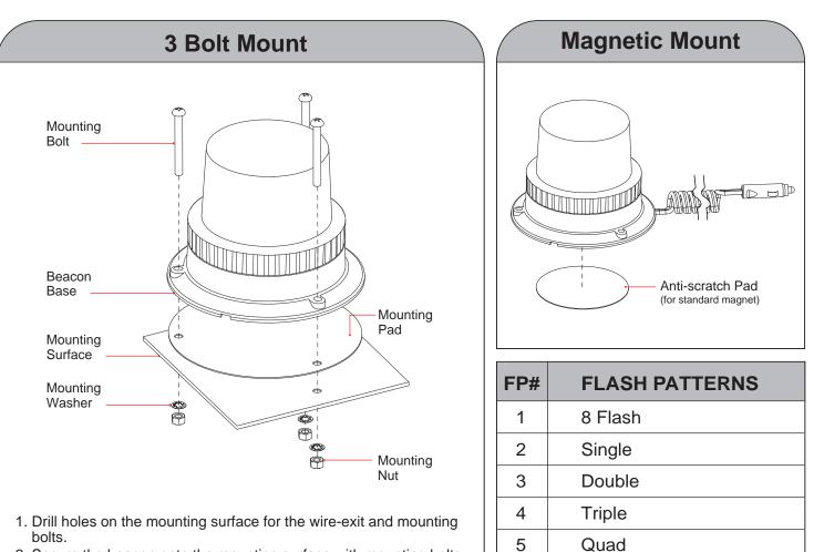
2. Secure the beacon onto the mounting surface with mounting bolts.
