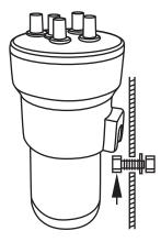
1) Trumpet & Compressor Mounting: Position each trumpet with open end facing down to prevent dirt & moisture from entering trumpet. Be sure to position the trumpets so that the supplied air hose will reach from each trumpet to the compressor. The compressor should be positioned so the outlets face upward. Drill holes and mount trumpets & compressor with the included hardware.
